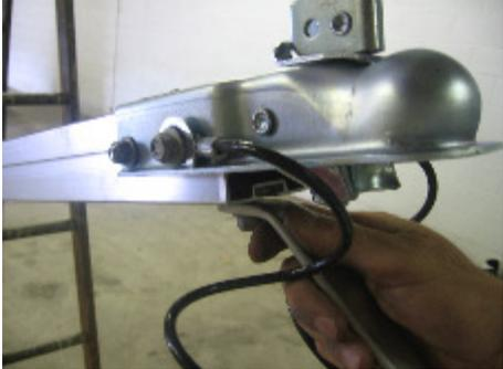
Slide the rear of the skid into the bottom slot in the front tongue section. Do not install the front of the skid yet.
