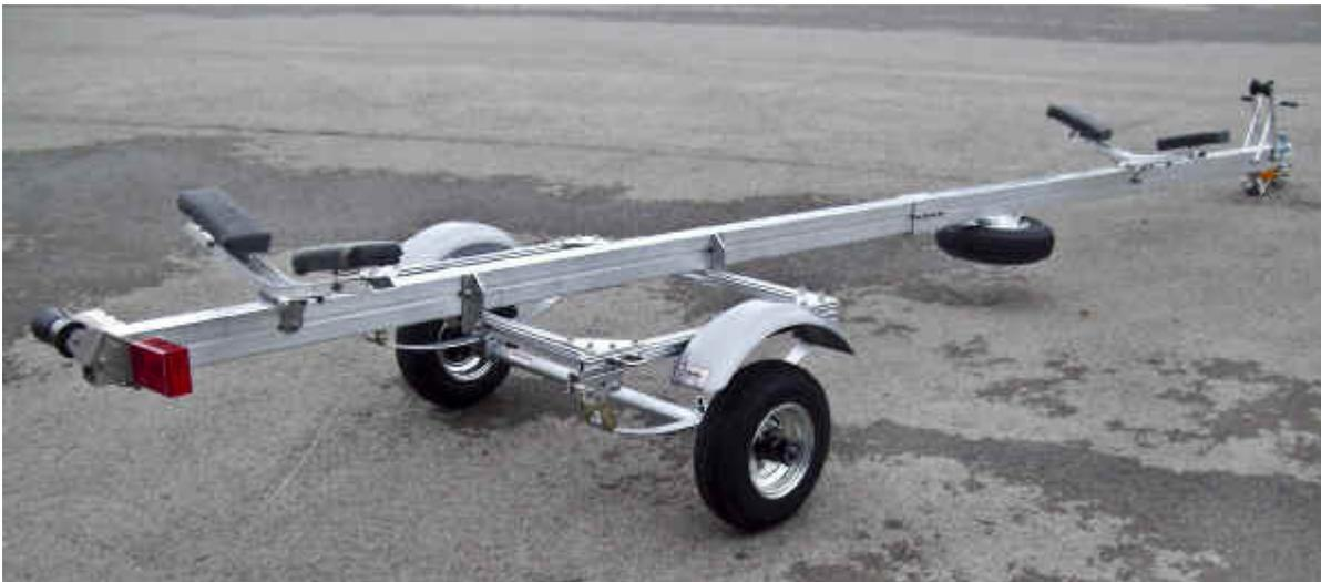
These are the steps, as shown in the SUT-series trailer assembly instructions, to mount the v support (skid). Reverse these steps in order to remove the v support, and install the spare tire carrier mount, then re-install the v support and running light bracket.
